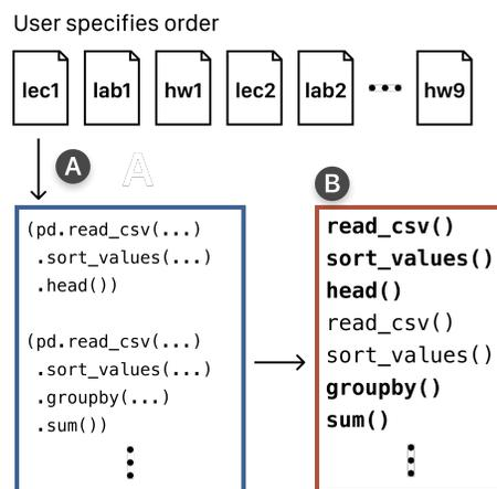
**Figure 2.** To use Codehound, users specify the order that each piece of content (e.g., a lecture, lab, or homework) is presented in the course. A) Codehound reads in instructional code in the same order it appears in the course. B) Codehound parses the code and extracts each function call in order of appearance (newly-encountered functions are shown in bold).
